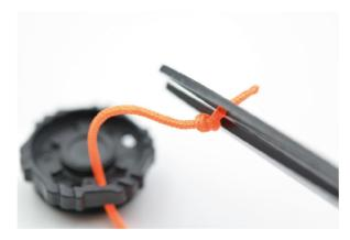
06 • Trim and singe the end of the rope so the knot is as small as possible.
