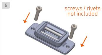
Install female base on planar surface using rivets or screws. Hole diameter 4mm. Max head diameter 9mm.
