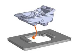
Position male connector into clip-in geometry.
