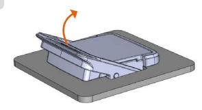
Check fit of cover and free movement of release trigger.
